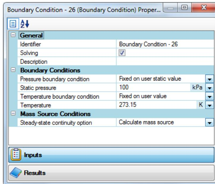
Figure 2: Specification of Static Boundary Conditions in Flownex<sup>®</sup>
