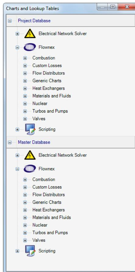
Figure 1: Project and Master Database in Flownex<sup>®</sup>
