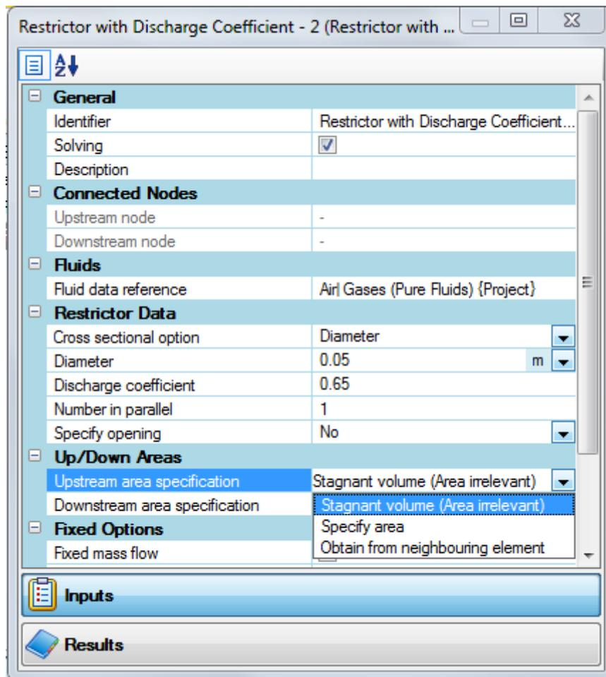
Figure 8: Upstream and Downstream Area Specification for the Restrictor with Discharge Coefficient in Flownex®
