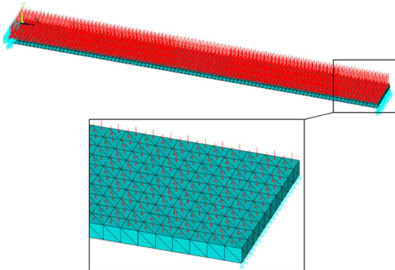
Figure 2. Tet Mesh One Element Through Thickness.
