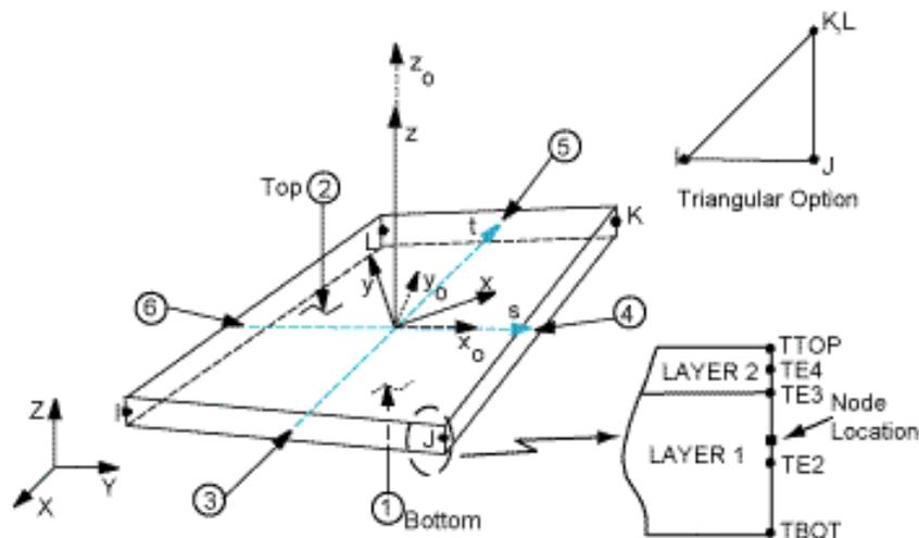
Figure 1. Shell 131 - 4 Node Layered Thermal Shell.
