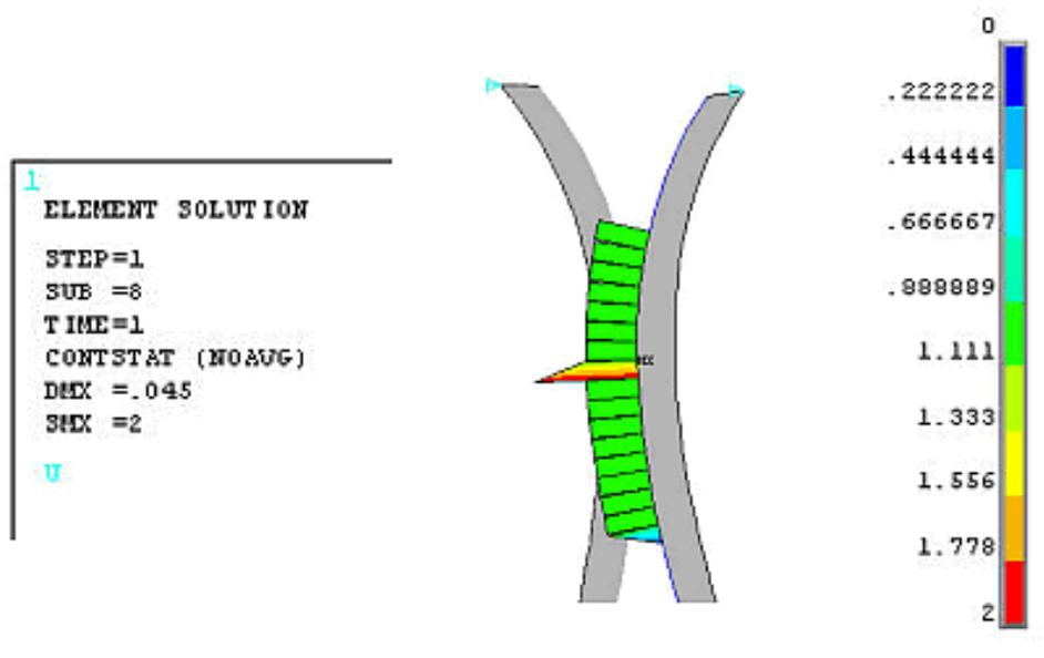
In the above depiction of contact status, it is clear that only a node or two is making contact during the solution.
