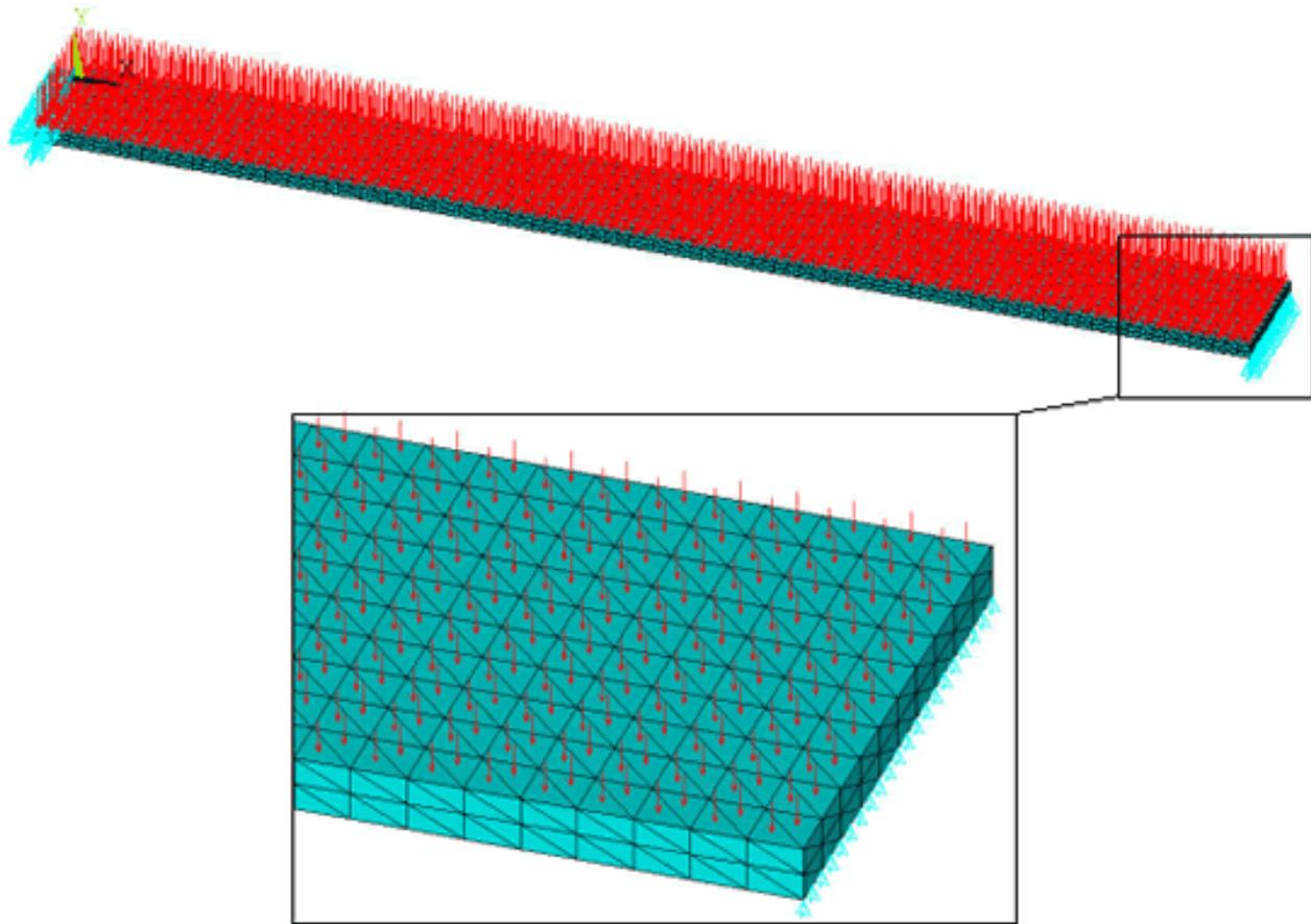
Figure 3. Tet Mesh Two Elements Through Thickness.
