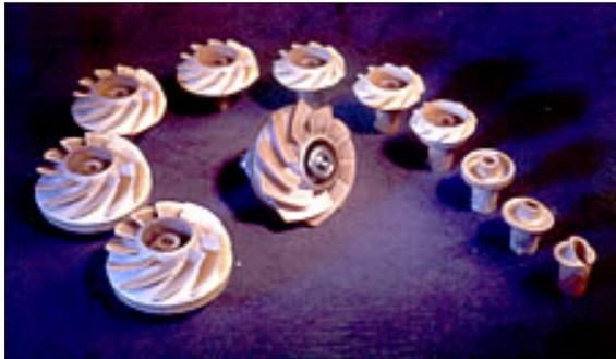
PADT put its rapid prototyping capabilities to a test recently by injection molding production-quality Ultem® fans for installation in fuel cells being tested and installed on operating automobiles.
