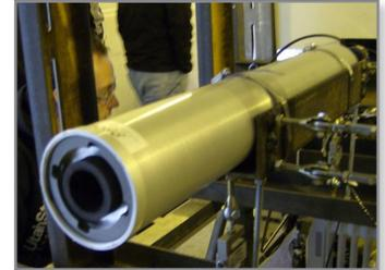
D-DART™ rocket motor mounted on the test cell
