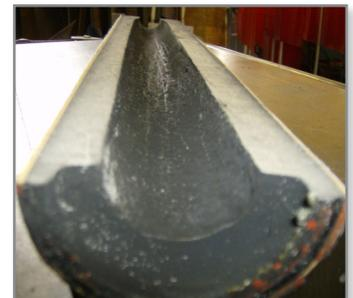
Sectioned ABS fuel grain after 10 second burn. Note no signs of the erosive burning characteristic of traditionally cast HTPB grains.
