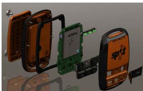
The entire product assembly was designed as an accurate 3D CAD model to enable faster downstream processes and meet stringent assembly and packaging demands.
