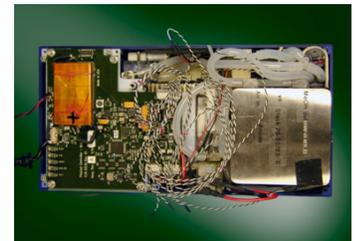
PADT worked with PolyFuel for 18 months to develop a fuel cell based, laptop power supply that was powered from a methanol fuel stock. We started with a blank sheet and developed a POC system that included the fuel cell stack, all of the custom components and controls, and was hybridized with a Lithium-ion battery pack. During that period Polyfuel was able to raise Venture Capital to develop their product.
