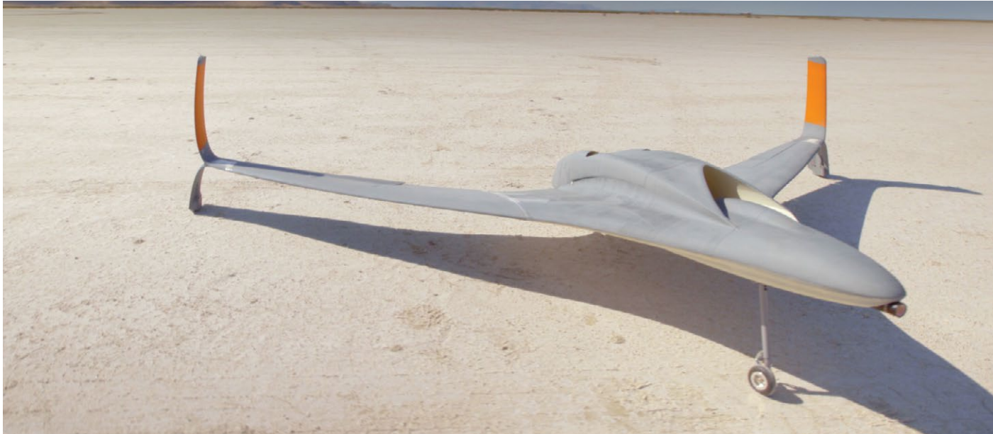
The jet-powered UAV developed by Aurora Flight Sciences is made with 34 parts; 26 of those are 3D printed.
