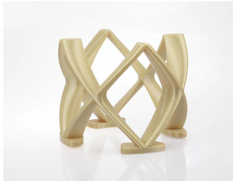
Additive manufacturing is the perfect fit for geometries shaped by topological optimization, producing shapes that would be difficult or impossible with conventional machine tools.
