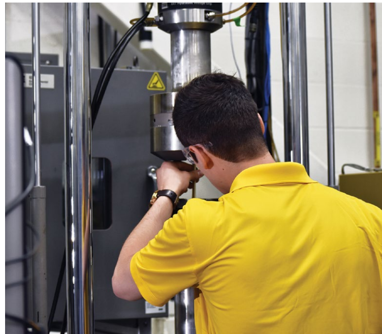
Tensile testing an ULTEM 9085 resin test coupon at the NIAR laboratory.
