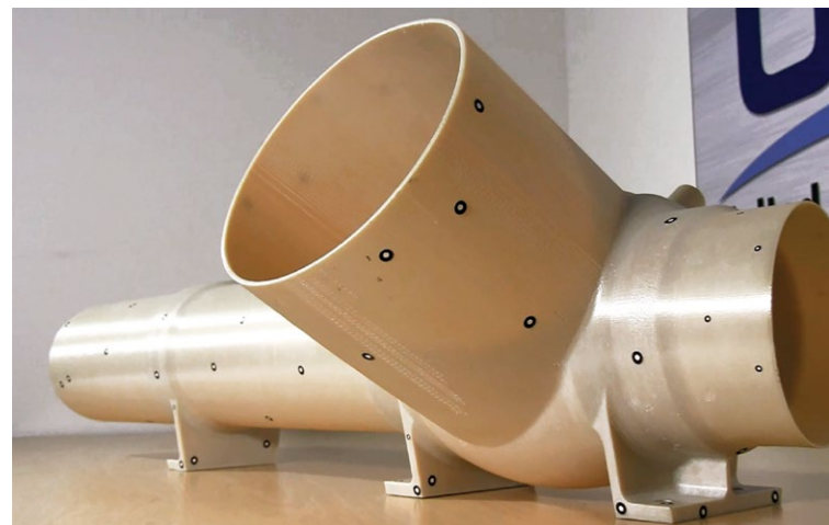
A portion of the additively manufactured ULA environmental systems duct used to cool avionics in the Atlas V payload fairing.
