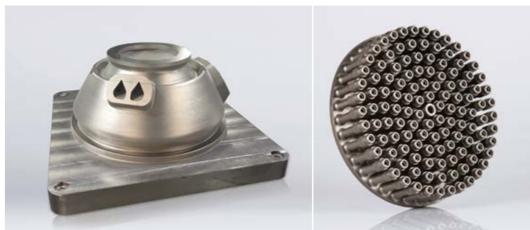
The additively manufactured injector head as all-in-one design (AiO) of a rocket engine with 122 injection elements is made from EOS NickelAlloy IN718. (left) The functional component of the all-in-one design: the baseplate. (right) (Source: EOS GmbH)
