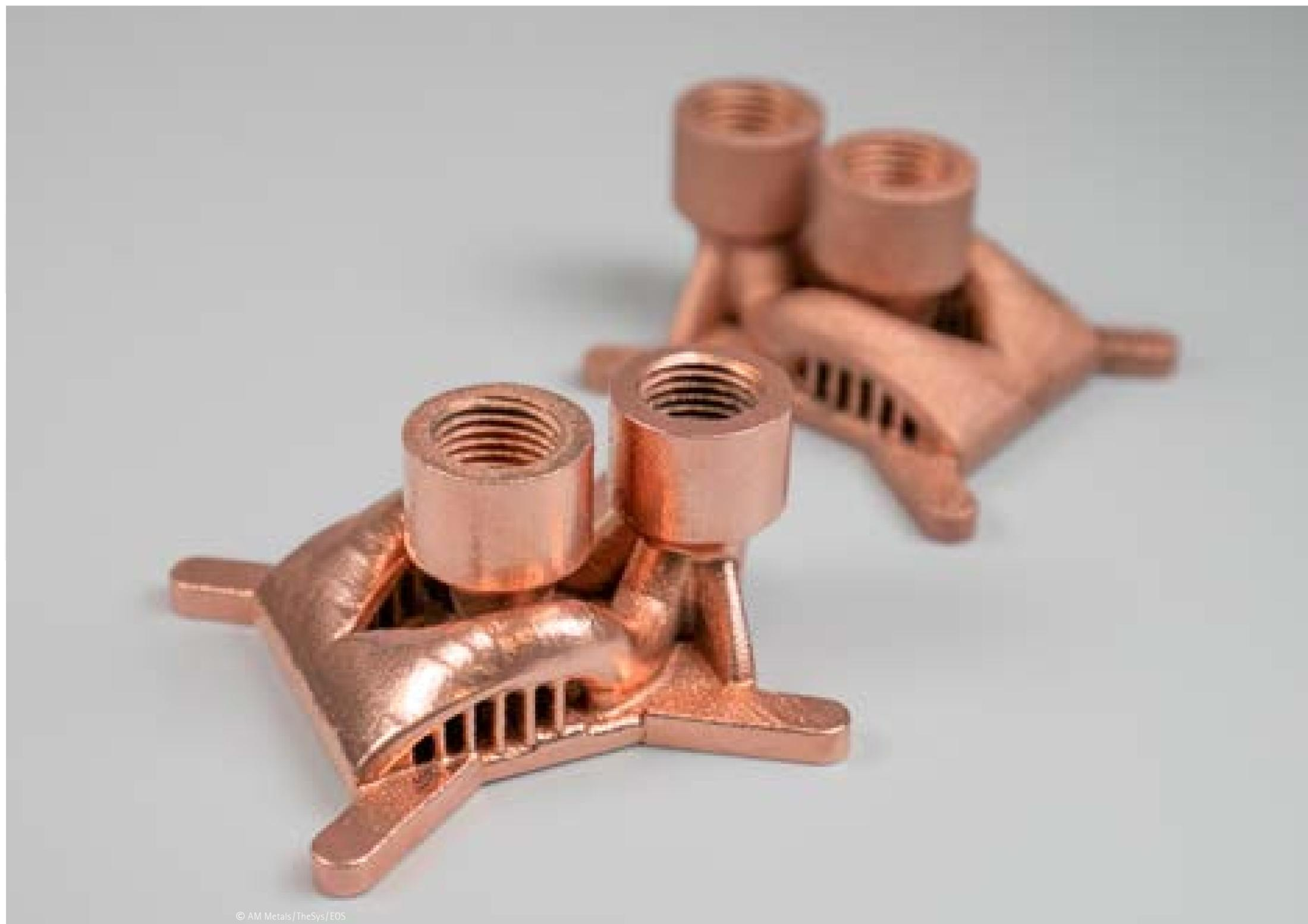
Figure 8: Innovated gaming CPU cooler optimized for 3D printing, manufactured on a standard EOS M 290 machine in pure copper from Elementum 3D
