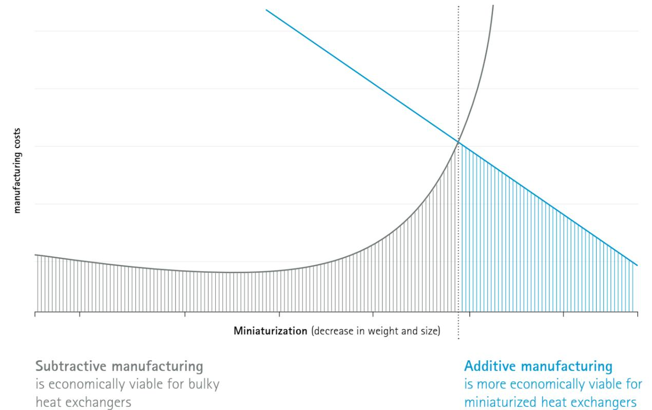
Figure 3: Delicate and complex components are where additive manufacturing shines, whereas massive parts with simple geometries are better suited for traditional subtractive manufacturing methods.
