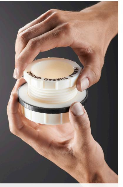
Threaded gauge prototype with male and female components
