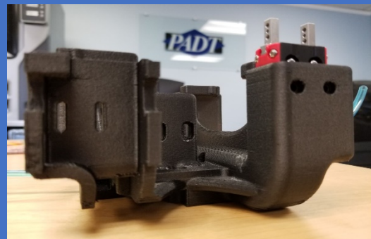
EOAT attached to 3D printed frame
