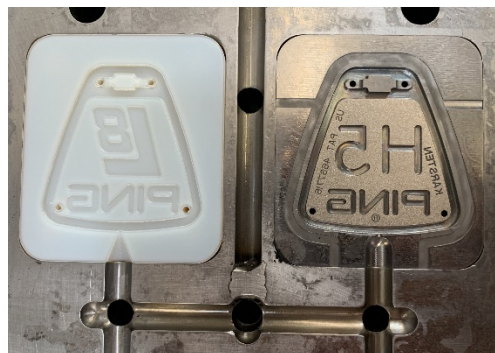
Fig. 2: A 3D printed injection mold compared to a more traditionally manufactured version of the same mold - Courtesy of PING
