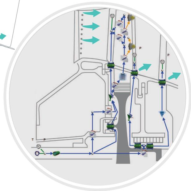
Flownex® includes a comprehensive rotating component flow library for analyzing the coolant rotational flow field inside the gas turbine engine, also referred to as the secondary air system. The Flownex® flow network approach leads to much faster and more cost-effective baseline designs for these systems since the number of expensive, detailed simulations are minimized.
