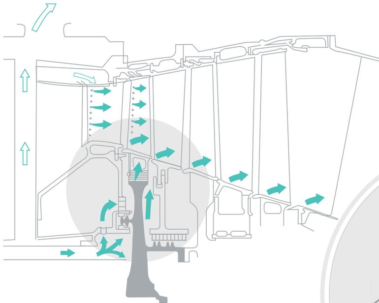
Model internal cooling system pressure, flow rate, power and heat transfer distribution with Flownex® to ensure effective film cooling on hot surfaces.
