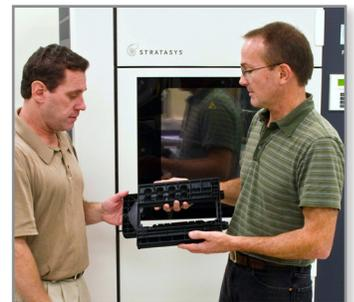
This prototype was created with the FDM process. It helped optimize the design for injection molding.
