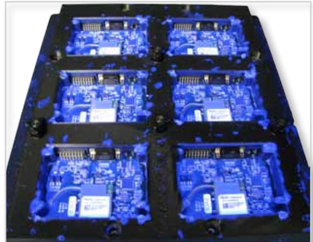
The application is jig and fixture making — which also includes gauges, organizational aids and other manufacturing devices. AM produces these tools by adding material in an automated, layer-by-layer process rather than removing material with a cutter or forming it in a mold.
