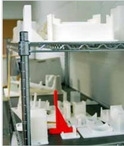
to make part replicas and CMM fixtures, Oreck creates its inspection plan and starts its CMM programming when a tooling order is released, not after samples are received. So, the QA department is ready and waiting for arrival of the first samples.
