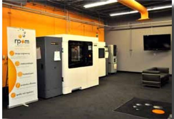
Three of rp+m's FDM additive manufacturing machines.
