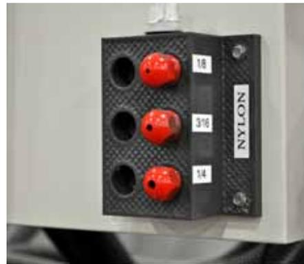
Injection molding nozzles organized in an additively manufactured work holder to make them accessible to press operators.
