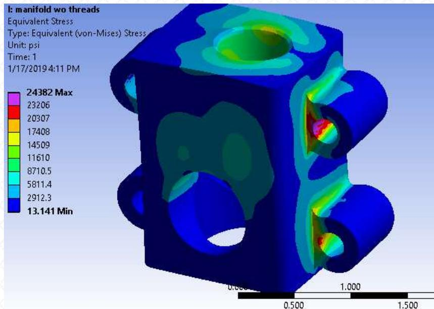
Simplified Model with all thread reactions applied to simplified thread surface
