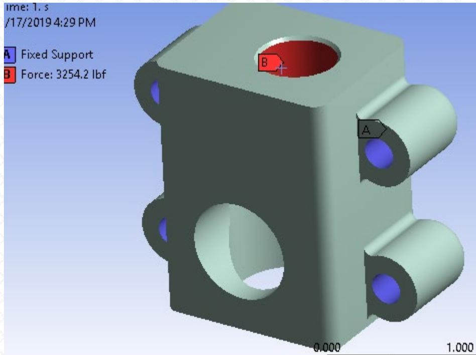
Simplified Model with radial thread load only:  $F_r = -3254.2$  lbf
