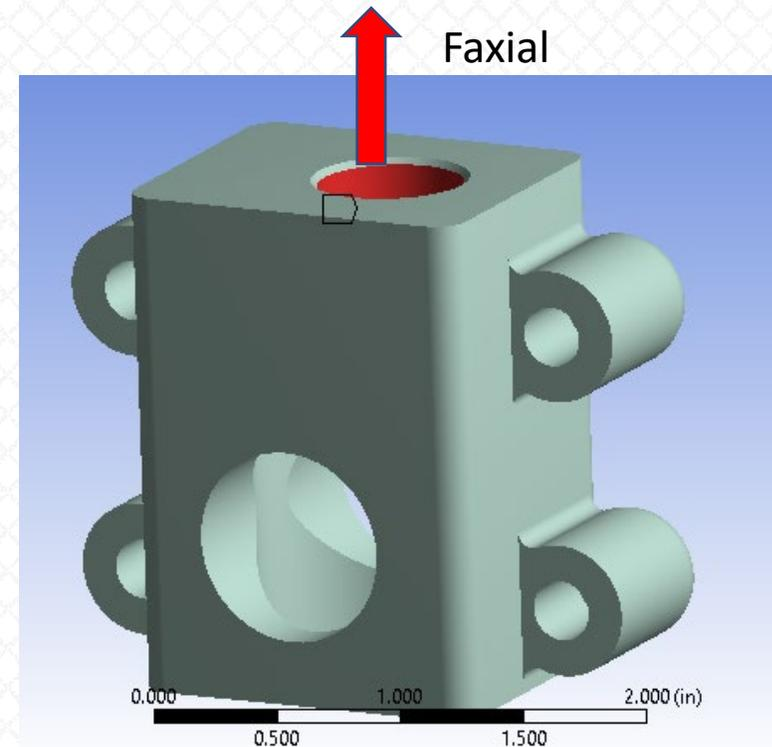
Case B: Simplified Model – Axial thread load
