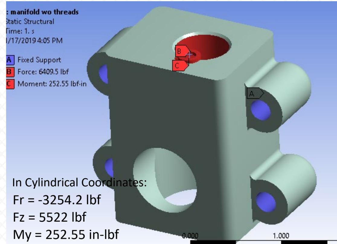
Case B: Simplified Model –Axial thread load
