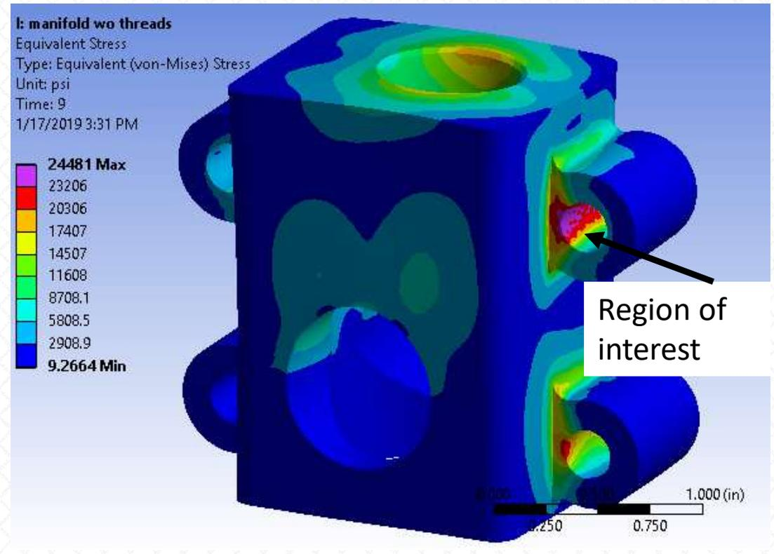
Case B: Simplified Model –Axial thread load
