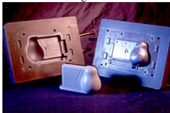
Figure 6. A large epoxy tool used to produce ABS parts. Cooling lines were used to help with thick section sink.
