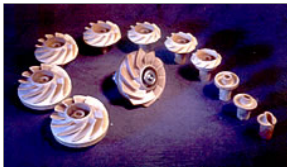
Figure 3. A series of short shots was used to warm the mold until it was ready to produce the Ultem® fan blades.
