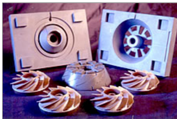
Figure 4. Pictured here, Ultem® blower parts with the RenCast epoxy inserts and mold halves in the center and background.
