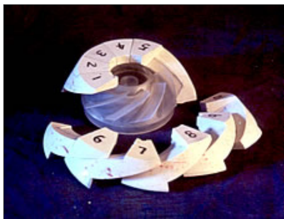
Figure 1. Mold forms were built for each fan rib using epoxy putty.
