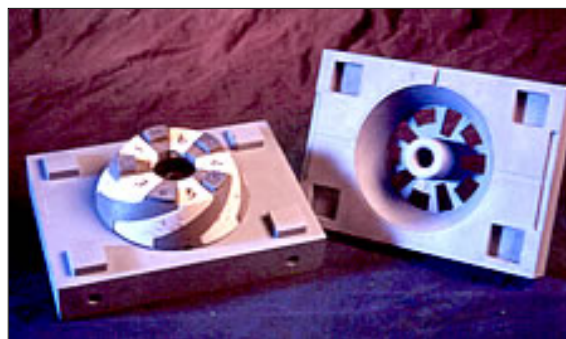
Figure 2. The two mold halves are pictured here with the even numbered mold inserts cast.
