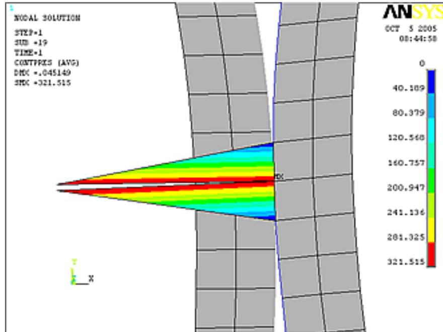
In ANSYS 10.0, a new keyoption was added for the 17X contact elements. As you recall from a previous [article](#), setting Keyopt 10=1 or 2 improved convergence by as much as 10 times over the default setting of 0.
