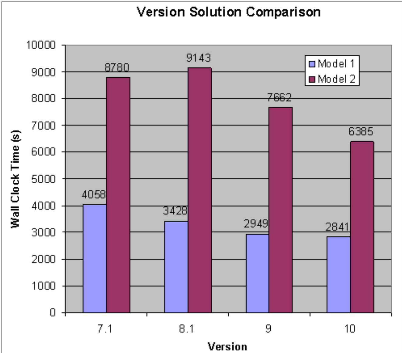
As you can see, 7.0 to 10.0 (pre-release) showed 27% and 30% speedups on the same hardware. Needless to say we verified that the amount of total creep strain calculated did not change. This is substantial if you do a lot of non-linear analysis.
